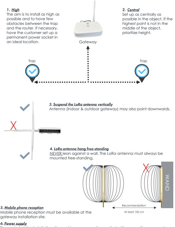
The socket at the installation site must be permanently supplied with power. If necessary, have a cable laid for this purpose.
